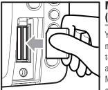
Inserting an MMC/SD into the Card Slot
